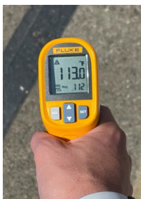
Surface temperatures before (113 degrees F) and after (104 degrees F) coating.
