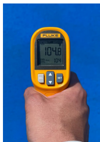
Surface temperatures before (113 degrees F) and after (104 degrees F) coating.
