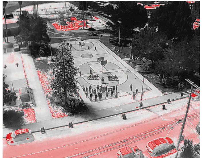
Thermal imagery of the basketball court after coating
