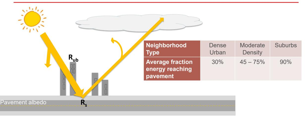
$R_{ub}$  = Incoming solar radiation in urban areas  $R_s$  = Reflected solar radiation from the pavement surface
